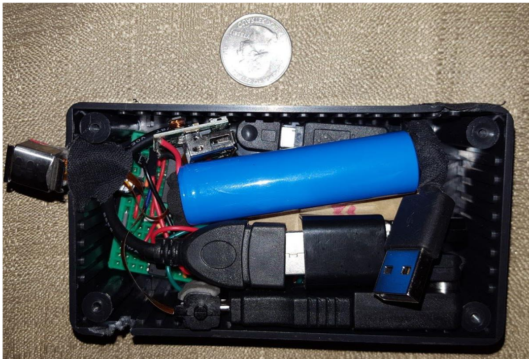
MagSpooF integrated with Raspberry zero
